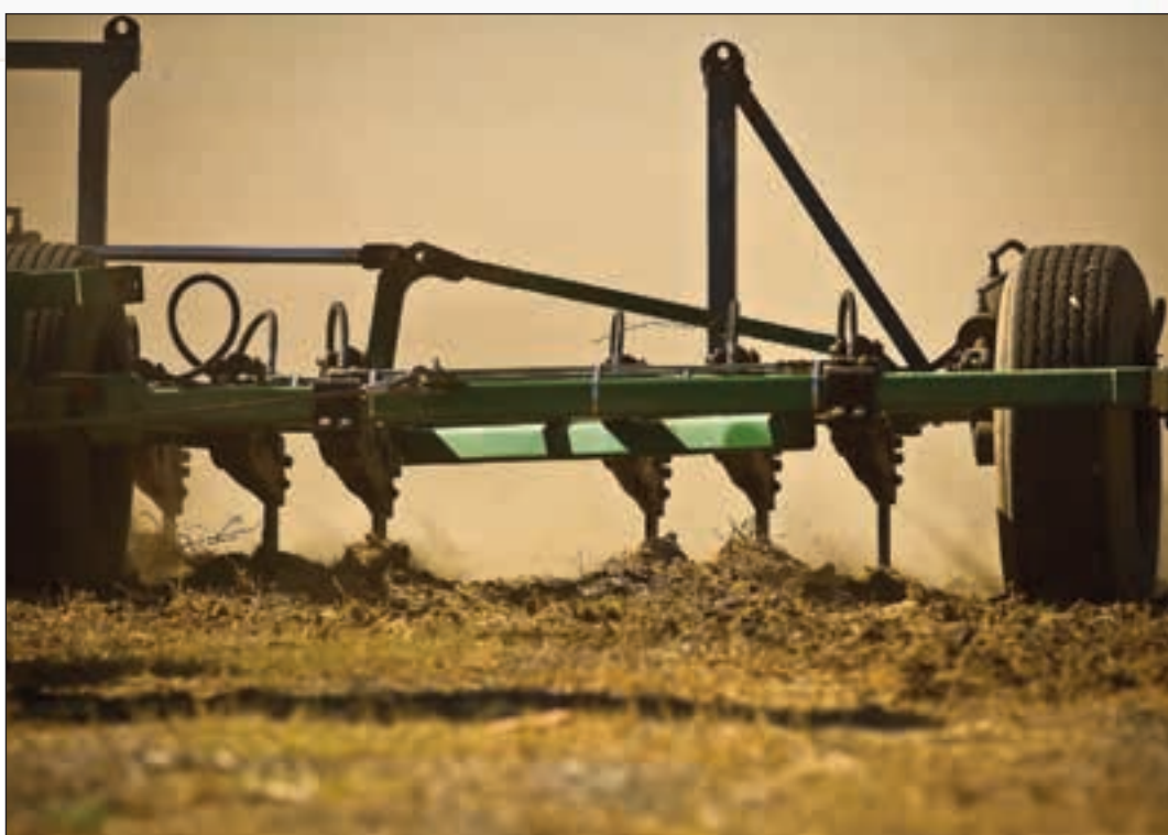
■ DEEP RIPPING... GRDC soils and nutrition manager — south, Stephen Loss, said strategic deep ripping is designed to ameliorate subsoil layers compacted by machinery traffic or natural cementation. PHOTO: GRDC
